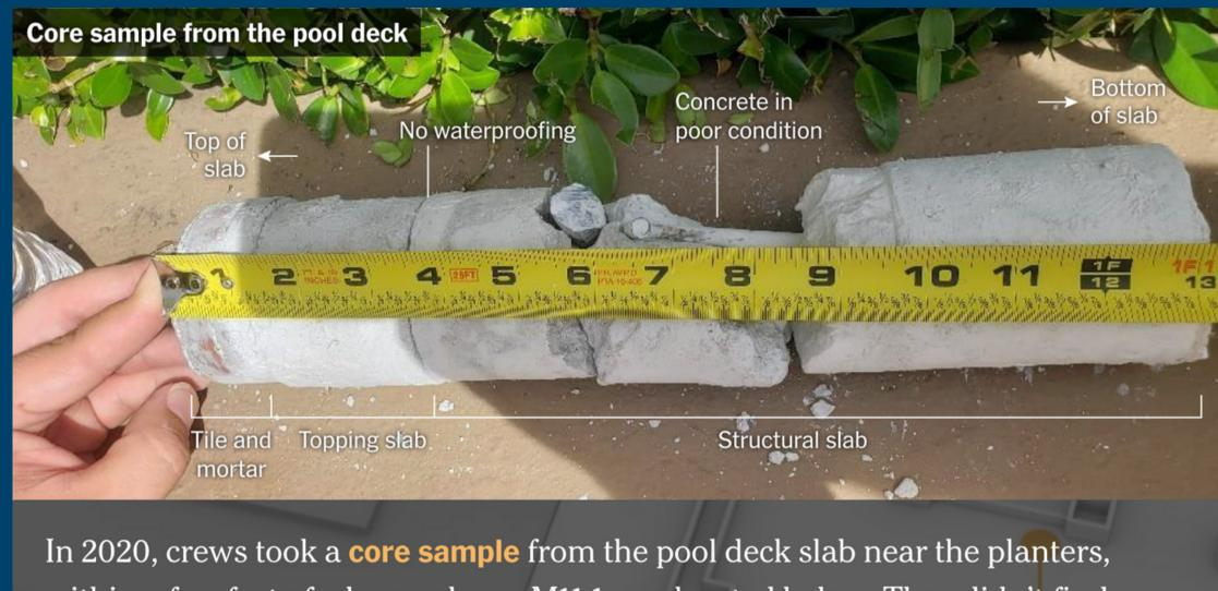
In 2020, crews took a **core sample** from the pool deck slab near the planters, within a few feet of where column M11.1 was located below. They didn't find any original waterproofing, and the concrete appeared to crumble away from the steel reinforcement inside the sample.
